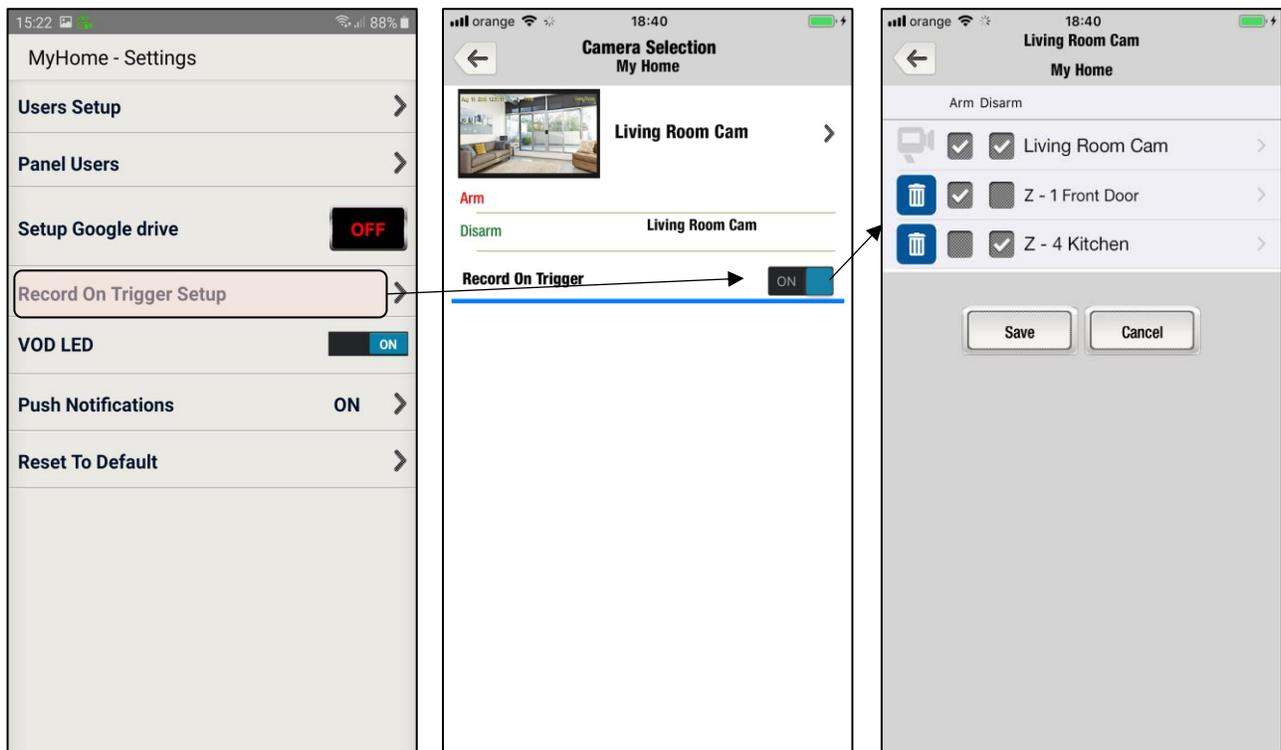
Allows enabling camera record based on an external trigger (e.g., Motion sensor from Zone 003 has triggered (motion detected)).
