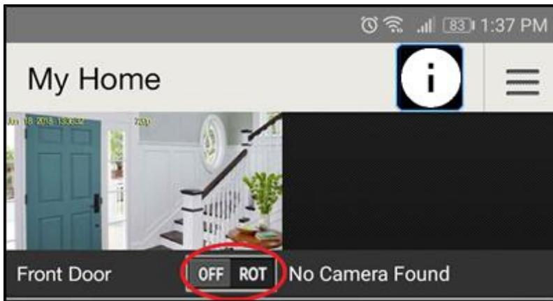
When the ROT button is pressed for a longer period of time, a new window opens, showing the video notification options.
